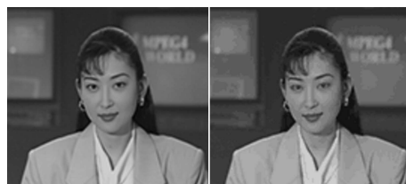
FIGURE 16. Akiyo reconstruction detail using AVGS - PSNR = 38db - d = 9 . Left: original, right: reconstruction.
