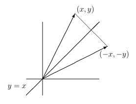
$F_{(1,1)}(x,y) = (-x,-y)$ Reflection about the line y = x
